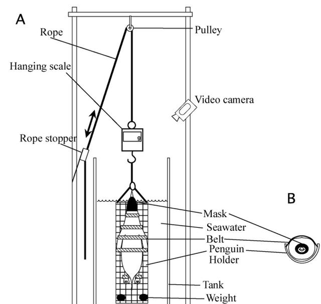
**Fig. 2 Schematic diagram of construct for underwater mass measurements**
